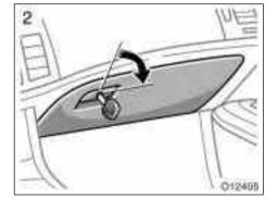
2. After closing the glove box lid, insert the master key (vehicles with key cylinder-type ignition switch) or mechanical key (vehicles with smart key system) and turn it clockwise to safeguard the lock release switch.
