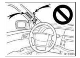
• Do not attach a microphone or any other device or object around the area where the curtain shield airbag activates such as on the windshield glass, side door glass, front and rear pillars, roof side rail and assist grips. When the curtain shield airbag inflates, the microphone or other device or object will be thrown away with great force or the curtain shield airbag may not activate correctly, resulting in death or serious injury.
