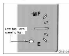
If the fuel tank is completely empty, the malfunction indicator lamp comes on. Fill the fuel tank immediately.
