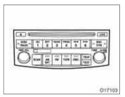
Type 3: AM-FM radio/compact disc player with changer (with cassette player and XM satellite radio<sup>\*</sup> controller)
