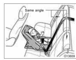
• When installing a child restraint system in the rear center position, adjust both seatbacks to the same angle. Otherwise, the child restraint system cannot be securely restrained and this may cause death or serious injuries in a collision.
