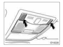
To turn on the front personal light, push the switch. To turn the light off, push the switch once again.
