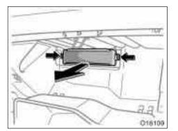
3. Remove the filter cover while pushing in both ends of the cover.
