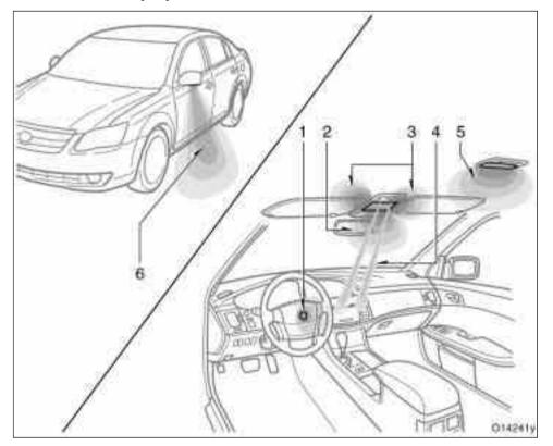
The following lights except the center console illumination and exterior foot lights will come on when any of the doors are opened. After all the doors are closed, the lights remain on for about 15 seconds before fading out.
