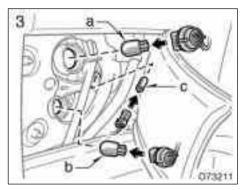
a: Rear turn signal light b: Stop/tail light c: Rear side marker light
