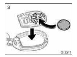
3. Put in a new transmitter battery with positive (+) side up. Install the circuit board into the transmitter case.
