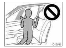
• Do not allow anyone to kneel on the passenger seat, facing the passenger's side door, since the side airbag and curtain shield airbag could inflate with considerable speed and force. Otherwise, he/she may be killed or seriously injured. Special care should be taken especially when you have a small child in the vehicle.
