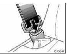
4. To remove the convertible seat, press the buckle release button and allow the belt to retract completely. The belt will move freely again and be ready to work for an adult or older child passenger.
