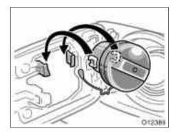
3. The removed cap can be stored on the back side of the fuel filler door.
