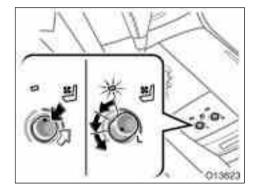
The front seat ventilator has two switches: one marked "L" (for driver's seat) and the other marked "R" (for front passenger's seat).
