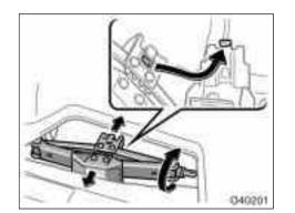
To store the jack, align the hole of the jack head with the vehicle hook. Turn the jack joint until the jack base fits securely with the vehicle body.
