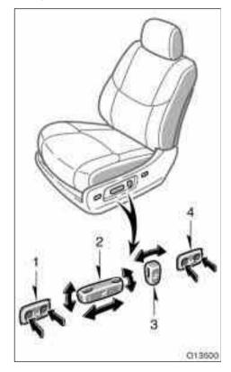
1. SEAT LEG SUPPORT ADJUSTING SWITCH (some models on driver's side)
