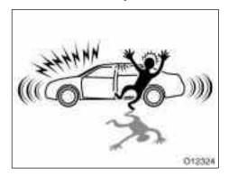
To deter vehicle theft, the system is designed to sound an alarm if any of the doors, trunk or hood is forcibly unlocked or the battery terminal is disconnected and then reconnected when the vehicle is locked.
