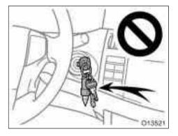
• Do not attach any heavy, sharp or hard objects such as keys or accessories to the ignition switch. The objects may restrict the SRS knee airbag inflation or be thrust into the driver's seat area by the force of the deploying airbag, thus causing a danger.
