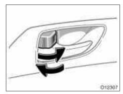
Closing the door with the lock knob in the lock position will also lock the door. Be careful not to lock your keys in the vehicle.
