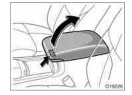
To access the rear console box, pull up the lock release lever while raising the rear console box lid.
