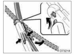
When the wipers no longer clean adequately, the wiper blades may be worn or cracked, requiring replacement.
