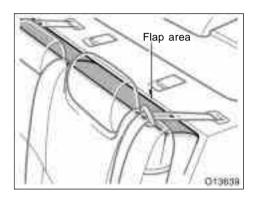
• Do not place objects on the flap area. Objects placed behind the rear seat may fall into the gap behind the seatback. If objects are left in the gap, the reclining seatback will not lock properly, leaving the seatback free to move. When the vehicle is in operation, moving seatbacks may cause injury.
