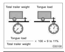
• The trailer cargo load should be distributed so that the tongue load is 9 to 11% of the total trailer weight, not exceeding the maximum of 45 kg (100 lb.). Never load the trailer with more weight in the back than in the front. About 60% of the trailer load should be in the front half of the trailer and the remaining 40% in the rear.
