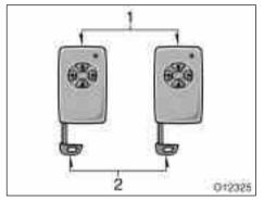
The key consists of an electronic key and a mechanical key. The mechanical key is for emergency use. If the electronic key does not operate, you can open the driver's door using the mechanical key.
