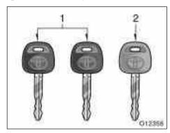
A transponder chip for engine immobilizer system has been placed in the head of the master and sub keys. These chips are needed to enable the system to function correctly, so be careful not to lose these keys. If you make your own duplicate key, you will not be able to cancel the system or start the engine.
