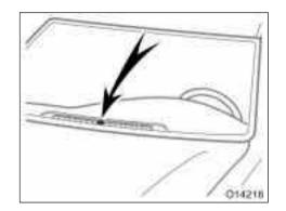
The automatic light control sensor is on the top of the center instrument panel.
