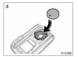
Put in a new battery with the positive (+) side up. Install the cover and insert the mechanical key into the transmitter.
