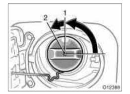
2. To remove the fuel tank cap, turn the cap counterclockwise by 90 degrees (to the pressure point 1), and then turn it an additional 30 degrees (to point 2). Pause slightly before removing it.
