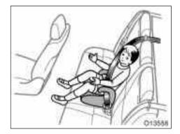
(C) BOOSTER SEAT INSTALLATION A booster seat must be used in forward-facing position only.
