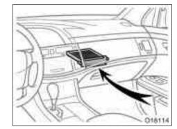
This air conditioning system has a high efficient air refiner filter which helps eliminate dust and pollen, thereby increasing your driving comfort.
