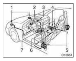
The seat belt pretensioner system consists mainly of the following components, and their locations are shown in the illustration.
