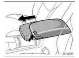
It is possible to use the rear console box lid as an armrest by moving it as shown in the illustration.
