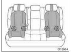
Lower anchorages for the child restraint systems complying with the FMVSS225 or CMVSS210.2 specifications are installed in the rear seat.
