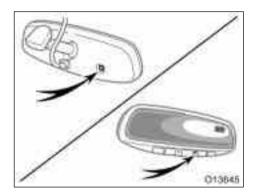
To ensure correct functioning of antiglare mirror sensors located on both side of the mirror, do not touch or cover the sensors with your finger or a piece of cloth, etc.
