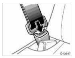
2. To remove the child booster seat, press the buckle release button and allow the belt to retract.
