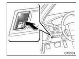
1. To open the fuel filler door, push the opener switch.
