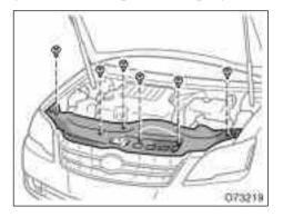
Remove the cover clips with a Phillipshead screwdriver and remove the covers.
