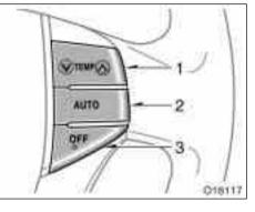
Some parts of the air conditioning system can be adjusted using the switches on the steering wheel.
