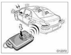
Unlocking operation (vehicles with smart key system)
