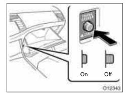
If you do not want to activate the trunk lid opener system, turn off the trunk opener main switch in the glove box. To turn it on, push in the trunk opener main switch again.
