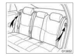
Seat belt comfort guides are stored in the both pockets on the sides of the rear seatback.
