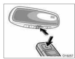
3. Simultaneously press and hold the hand-held garage transmitter button along with the selected HomeLink<sup>®</sup> button.
