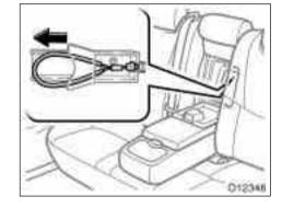
2. Pull the loop of wire to unlock the trunk lid.
