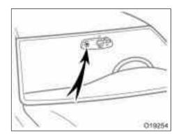
The compass sensor is in the inside rear view mirror.
