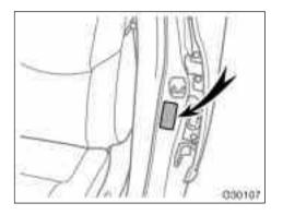
• The gross vehicle weight must not exceed the Gross Vehicle Weight Rating (GVWR) indicated on the Certification Label. The gross vehicle weight is the sum of weights of the unloaded vehicle, driver, passengers, luggage, hitch and trailer tongue load. It also includes the weight of any special equipment installed on your vehicle.
