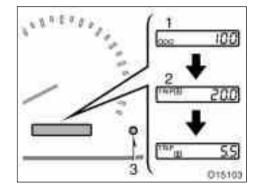
This meter displays the odometer and two trip meters when the ignition switch is set at ON.
