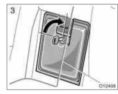
3. After closing the door located behind the rear seat armrest, insert the master key (vehicles with key cylinder-type ignition switch) or mechanical key (vehicles with smart key system) and turn it clockwise to lock the door.
