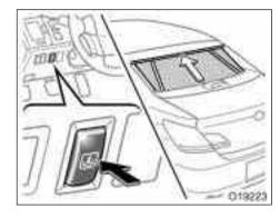
To raise the rear electric sunshade, push the switch. To lower the sunshade, push the switch again.
