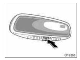
5. Test the operation of the HomeLink<sup>®</sup> by pressing the newly programmed button. If programming a garage door opener, check to see if the garage door opens and closes.
