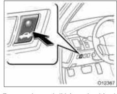
To open the trunk lid from the driver's seat, push the trunk opener switch.
