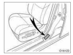
The air conditioning filter information label is placed as shown and indicates that a filter has been installed.
