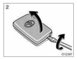
2. Using a flathead screwdriver or equivalent, open the transmitter case.
