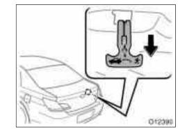
If a person is locked in the trunk, he/she can pull down the phosphorescent strap on the inside of trunk lid to open the trunk lid.
