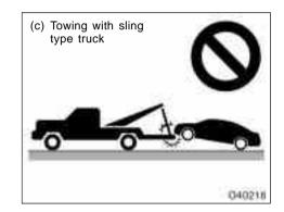
(c) Towing with sling type truck
