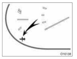
If a buzzer sounds and the smart key system warning light comes on for 5 seconds when pressing the "ENGINE START STOP" switch, this indicates that the key is not in the vehicle.
