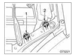
Vertical movement adjusting bolt 1
