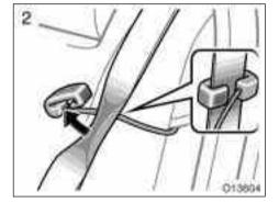
2. Pinch the two edges of the shoulder belt for the rear seat outside position with your fingers and slide the belt past the slot of the guide as shown above. At this time, the elastic cord must be behind the seat belt.
