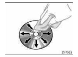
To clean a compact disc: Wipe it with a soft, lint-free cloth that has been dampened with water. Wipe in a straight line from the center to the edge of the disc (not in circles). Dry it with another soft, lint-free cloth. Do not use a conventional record cleaner or anti-static device.
