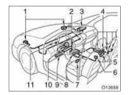
The SRS front airbag system mainly consists of the following components, and their locations are shown in the illustration.
