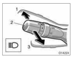
**High-Low beams**—For high beams, turn the headlights on and push the lever away from you (position 1). Pull the lever toward you (position 2) for low beams.
