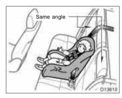
• When installing a child restraint system in the rear center position, adjust both seatbacks to the same angle. Otherwise, the child restraint system cannot be securely restrained and this may cause death or serious injuries in a collision.
