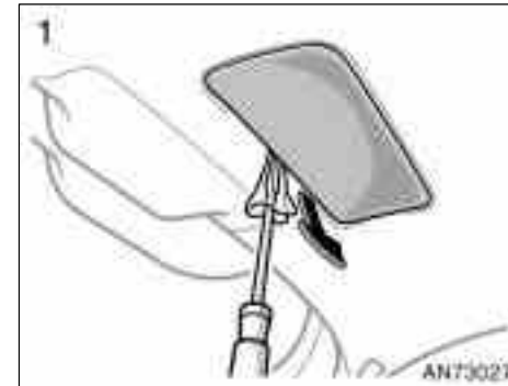
Remove the cover with a flat-bladed screwdriver which is wrapped with a cloth.
