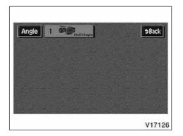
The angle can be selected for discs that are multi-angle compatible when the """" mark appears on the screen. Each time you push the "Angle" switch, the angle changes. The angle number which you can select will appear on the screen.
