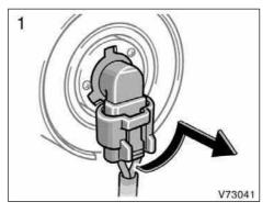
1. Open the hood. Turn the bulb base counterclockwise to the front of the vehicle as shown.
