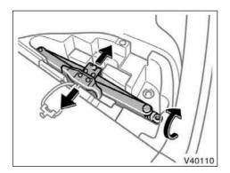
To store the jack, rotate the jack joint until the jack is firmly secured.
