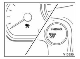
The SRS warning light and "AIRBAG OFF" indicator light will come on if there is a malfunction in the front passenger occupant classification system.
