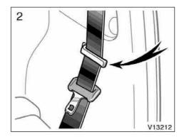
2. Make sure the outer seat belts passes through the hangers when folding the second seat.
