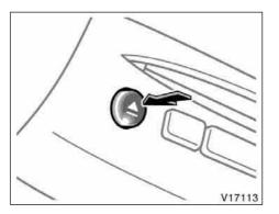
EJECTING THE DISC Push the "**≜**" button.
