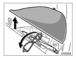
Before removing the jack, remove the right side deck board and unhook the tightening strap.
