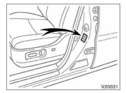
The vehicle identification number (VIN) is also on the Certification Regulation Label.
