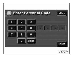
Push the number for the password and the "Enter" switch. The "Select Restriction Level" screen will appear.
