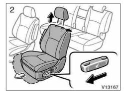
2. Remove the head restraint. Push the seat position adjusting switch forward to slide the front seat to the front-most position.
