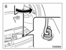
6. Threading the jack handle through the adapter socket, turn the jack handle counterclockwise. Continue until the spare tire is lowered completely to the ground.
