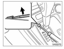
If you cannot shift the selector lever out of the "P" position to other positions even though the brake pedal is depressed, use the shift lock override button as follows:
