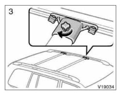
3. In order to fix the cross rails to the appropriate length, turn the upper knobs clockwise after tightening all of the side knobs.
