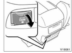
This power outlet is designed for use as a power supply for the audio device connected to the input terminal adapter.
