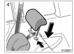
4. Replace the head restraint and lift it up to the uppermost lock position.
