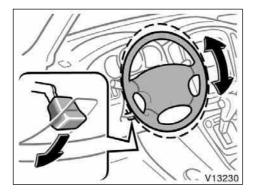
To change the steering wheel angle, hold the steering wheel, push down the lock release lever, tilt the steering wheel to the desired angle and return the lever to its original position.
