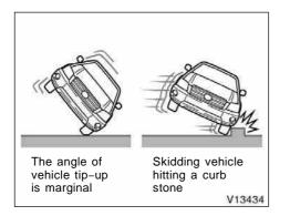
The SRS curtain shield airbags may inflate if the angle of vehicle tip-up is marginal or if the skidding vehicle's tires hit a curb stone laterally as shown in the illustration.
