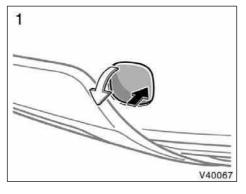
1. Remove the front towing eyelet cover on the front bumper by pushing the outside of the cover.
