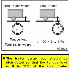
weight, not exceed the following. 2AZ-FE engine Without towing package 68 kg (150 lb.) With towing package 136 kg (300 lb.) 3MZ-FE engine Without towing package 90 kg (200 lb.) With towing package
