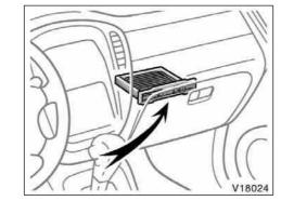
The air conditioning filter is behind the glove box.
