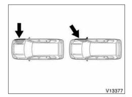
The SRS side airbags may not activate if the vehicle is subjected to a collision from the side at certain angles, or a collision to the side of the vehicle body other than the passenger compartment as shown in the illustration.
