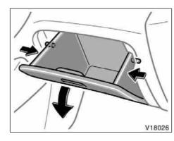
2. Open the glove box and push each side of the glove box to disconnect the claws.
