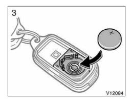
3. Put in a new transmitter battery with positive (+) side up.
