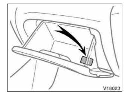
The air conditioning filter information label is placed in the glove box as shown and indicates that a filter has been installed.
