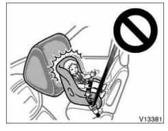
• Never install a rear-facing child restraint system on the front passenger seat even if the "AIRBAG OFF" indicator light is illuminated. In the event of an accident, the impact of the rapid inflation of the front passenger airbag could cause death or serious injury to the child if the rear-facing child restraint system is installed on the front passenger seat.
