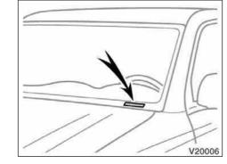
The vehicle identification number (VIN) is the legal identifier for your vehicle. This number is on the left top of the instrument panel, and can be seen through the windshield from outside.
