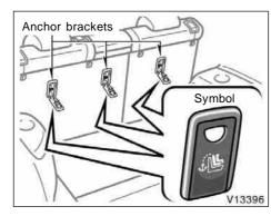
Use the anchor brackets behind the second seat seatbacks to secure the top strap.
