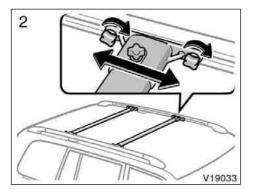
2. Slide the cross rails to the appropriate position for loading the luggages and turn the side knobs clockwise to tighten the cross rails securely.
