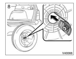
8. Remove the holding bracket. Vehicles with aluminium wheels— Remove the spare tire cover.
