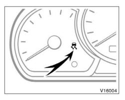
If the vehicle is going to skid during driving, the slip indicator light blinks and an alarm sounds intermittently. Special care should be taken while driving.
