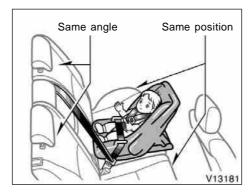
• When installing a child restraint system in the second seat center position, adjust both seat cushions to the same position and align both seatbacks at the same angle. Otherwise, the child restraint system cannot be securely restrained and this may cause death or serious injuries in a collision.
