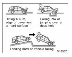
The SRS front airbags may also deploy if a serious impact occurs to the underside of your vehicle. Some examples are shown in the illustration.
