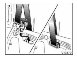
2. To stow the seat belt, insert the tabs into the slot as shown above. Make sure the tabs are securely locked in the slot.
