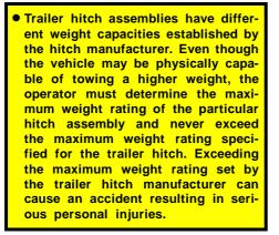
• The gross vehicle weight must not exceed the Gross Vehicle Weight Rating (GVWR) indicated on the Certification Label. The gross vehicle weight is the sum of weights of the unloaded vehicle, driver, passengers, luggage, hitch and trailer tongue load. It also includes the weight of any special equipment installed on your vehicle.
