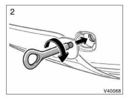
2. Use the front towing eyelet in the luggage compartment. Secure it to the hole on the bumper by turning clockwise. (For the towing eyelet location, see "-Required tools and spare tire" on page 338 in this Section.)
