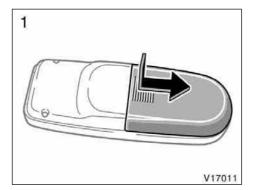
1. Remove the cover of the controller as shown.
