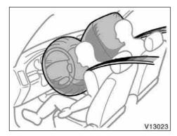
The SRS front passenger airbag will not activate if there is no passenger sitting in the front passenger seat. However, the front passenger airbag may deploy if luggage is put in the seat, or the seat belt is buckled up, regardless of the presence of an occupant in the seat. (As for the front passenger occupant classification system, see "—Front passenger occupant classification system" on page 86 in this Section.)
