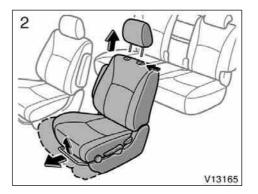
2. Remove the head restraint. Hold the center of the lever and pull it up. Then slide the front seat further forward than the front-most lock position.
