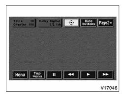
To turn on the selecting switch, push the " $\diamondsuit$ " switch.
