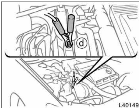
Connecting point for 1MZ-FE and 3MZ-FE engines
