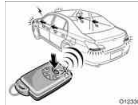
Locking operation (vehicles with smart key system)
