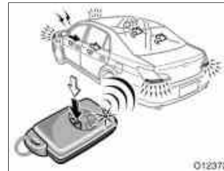
Unlocking operation (vehicles with smart key system)
