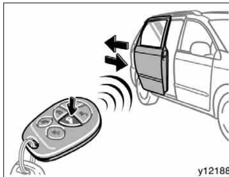
Right side power sliding door (type B)
