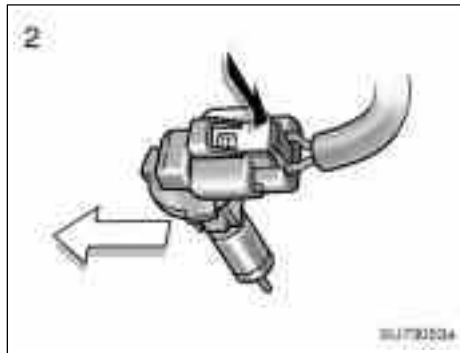
2. Pull the bulb out of the bulb base. If the connector is tight, wiggle it.
