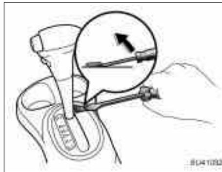
If you cannot shift the selector lever out of “P” position even though the brake pedal is depressed, use the shift lock override button as follows:
