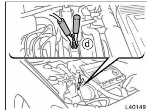
Connecting point for 1MZ-FE and 3MZ-FE engines
