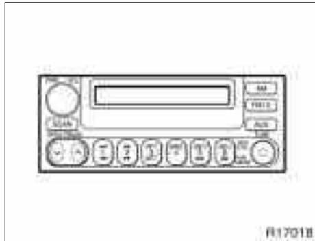
Type 1: AM-FM radio (with cassette and compact disc auto changer controllers)
