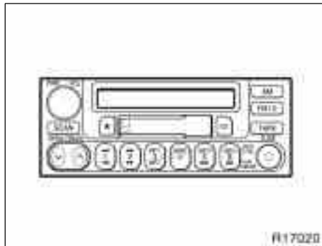
Type 2: AM-FM radio/cassette player (with compact disc auto changer controller)
