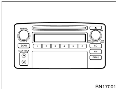
Type 1: AM-FM ETR radio/compact disc player (with cassette and compact disc auto changer controllers)
