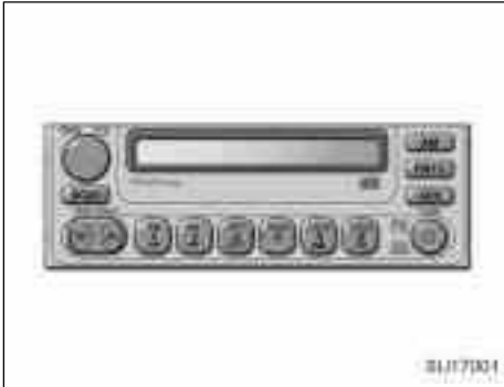
Type 1: AM-FM ETR radio (with cassette and compact disc auto changer controller)
