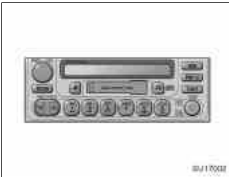
Type 2: AM-FM ETR radio/cassette player (with compact disc auto changer controller)
