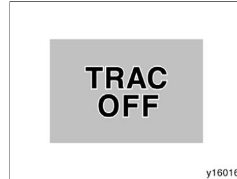
“TRAC OFF” indicator/warning light
