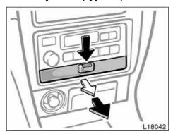
To use the box, push down the knob and pull it out completely.
