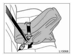
Run the lap and shoulder belt through or around the infant seat following the instructions provided by its manufacturer and insert the tab into the buckle taking care not to twist the belt. Keep the lap portion of the belt tight.
