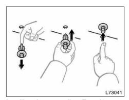
Installing the cover clips (Type A)
