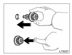
Installing the cover clips
