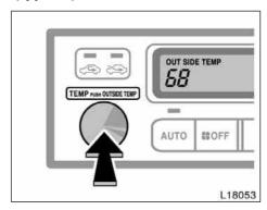
The outside temperature gauge indicates the outside air temperature when you push the "TEMP" selector button.
