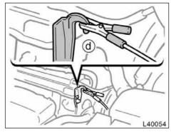
Connecting point for 5S-FE engine
