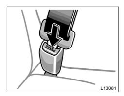
To remove the child restraint system, press the buckle-release button and allow the belt to retract.
