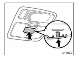
When the garage door opener transmitter is properly installed, you can operate the transmitter by pushing the center panel of the cover.
