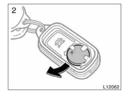
2. Remove the discharged transmitter battery.
