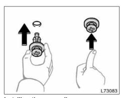
Installing the cover clips
