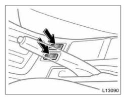
To turn on the seat heater, push the switch.
