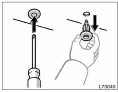
Removing the cover clips (Type A)
