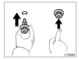
Installing the cover clips (Type B)
