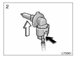
2. Unplug the connector while depressing the lock release.
