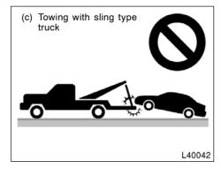
(c) Towing with sling type truck
