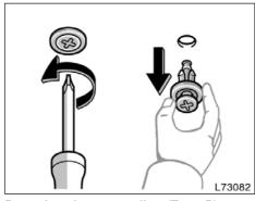
Removing the cover clips (Type B)
