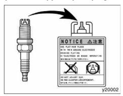
Your engine is fitted with twin ground electrode platinum-tipped spark plugs.
