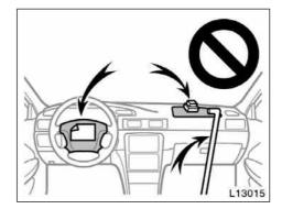
• Do not put objects or your pets on or in front of the dashboard or steering wheel pad that houses the front airbag system. They might restrict inflation or cause death or serious injury as they are projected rearward by the force of deploying airbags. Likewise, the driver and front passenger should not hold things in their arms or on their knees.
