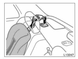
Follow the procedure below for a child restraint system that uses of a top strap to ensure the system. Follow all the installation instructions provided by its manufacturer.
