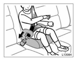
Sit the child on a booster seat. Run the lap and shoulder belt through or around the booster seat and child following the instructions provided by its manufacturer and insert the tab into the buckle taking care not to twist the belt.
