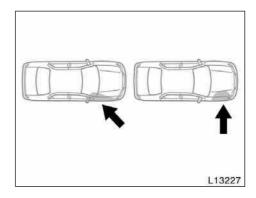
The SRS side airbag system may not activate if the vehicle is subjected to a collision from the side at certain angles, or a collision to the side of the vehicle body other than the passenger compartment as shown in the illustration.
