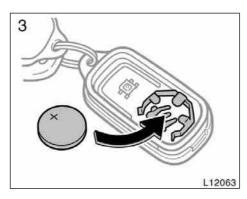
3. Put new transmitter battery with positive (+) side up.
