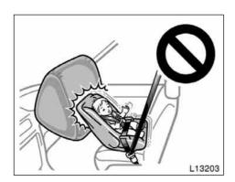
• Never put a rear-facing child restraint system on the front passenger seat because the force of the rapid inflation of the front passenger airbag can cause death or serious injury to the child.
