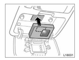
Place the transmitter with Velcro loop facing inside of box into the box. Make sure the transmitter button is located above button pins.
