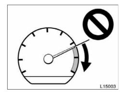
The tachometer indicates engine speed in thousands of rpm2(revolutions per minute). Use it while driving to select correct shift points and to prevent engine lugging and over-revving.
