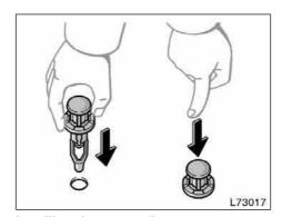
Installing the cover clips
