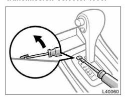
If you cannot shift the selector lever out of "P" position to other positions even though the brake pedal is depressed, use the shift lock override button as follows:
