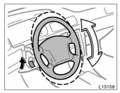
To change the steering wheel angle, hold the steering wheel, pull up the lock release lever, tilt the steering wheel to the desired angle and release the lever.
