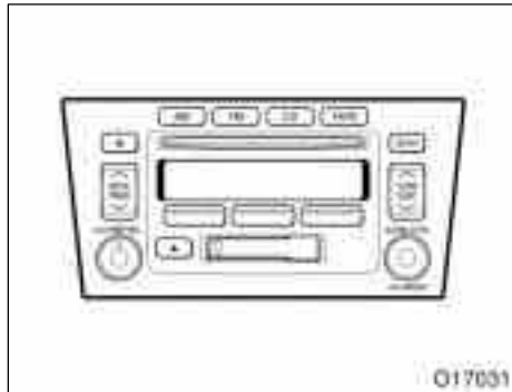
Type 1: AM-FM ETR radio/cassette player/ compact disc player/compact disc auto changer controller
