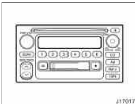
Type 2: AM-FM ETR radio/cassette player/compact disc player/compact disc auto changer controller
