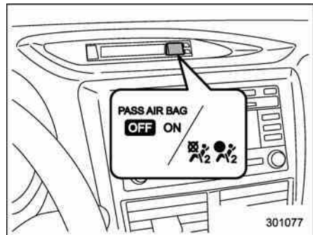
ON / : Front passenger's frontal airbag ON indicator OFF / : Front passenger's frontal airbag OFF indicator
