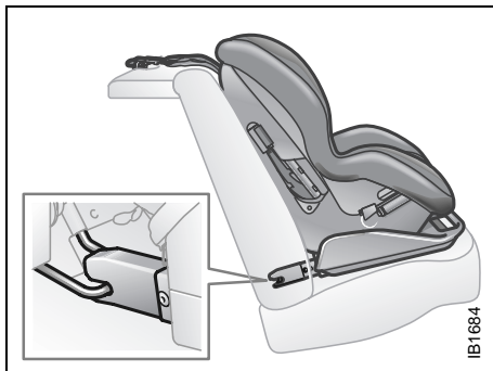
Rigid 2-point lower attachment with top tether
