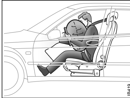
Inflated airbag (driver side) Inflation and deflation together take less than 0.1 second.
