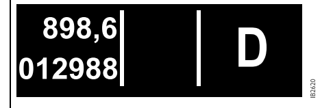
Indication of gear position on main instrument panel
