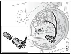
Parking-light bulb (cars with halogen low beam)
