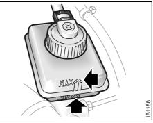
Brake and clutch-fluid reservoir
