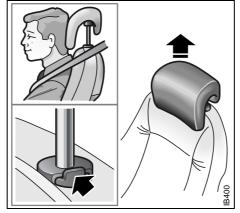
The head restraint can be raised or lowered and is adjustable in various positions.
