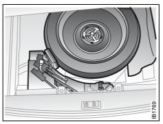
The car's ground clearance is reduced with the compact spare fitted. Note that only one compact spare wheel may be used at any time. Take care not to hit the curb and do not fit snow chains. Leave the wheel cover off, so that the warning text is readily visible.
