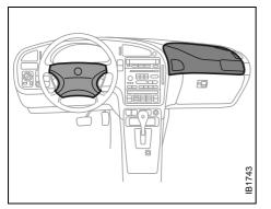
Accessories and other equipment must not be fitted to the surfaces marked as these are where the airbags inflate in the event of a crash.
