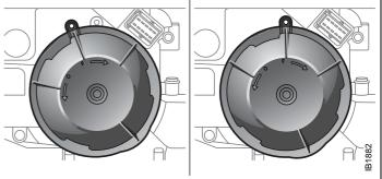
Make sure the cover is correctly fitted before locking it in place
