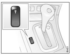
Switch for operation of central locking
