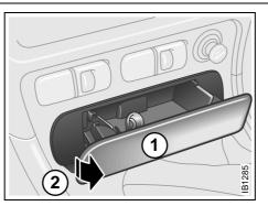
*Front ashtray* 1 Press soft to open/close 2 Pull out one side at an angle
