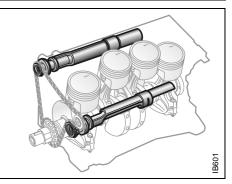
Balance shafts, 4-cyl. engine
