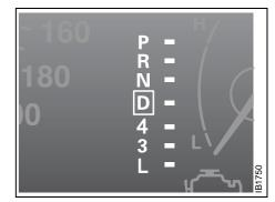
Selector-lever indicator on main instrument panel
