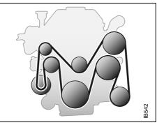
Routing of the Poly-V-belt: 4-cylinder engine
