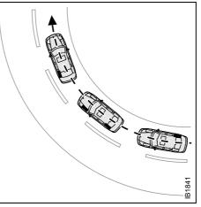
Increased stability with ESP. The system applies the brakes to the wheels as shown to prevent the car from skidding
