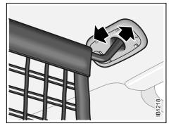
Attaching the cargo net to the roof
