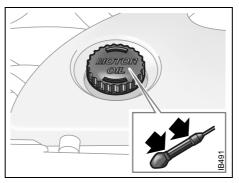
Engine-oil filler cap and dipstick, 4-cylinder engine
