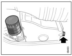
Drain plug and oil filter, 4-cylinder engine
