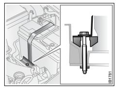
Correct position for battery clamp
