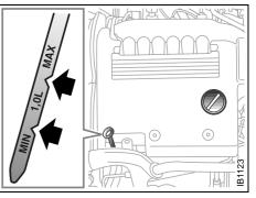
Engine-oil dipstick and filler cap, 3.0t V6
