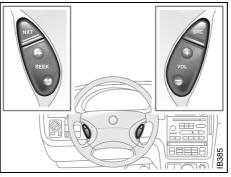
Audio System controls on steering wheel
