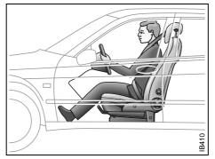
Correctly positioned safety belt
