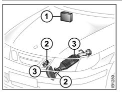
Oxygen-sensor-controlled injection system 1 Engine control module
