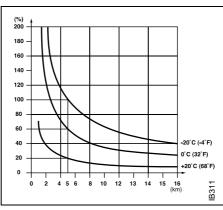
Percentage increase in fuel consumption of engine starting from cold compared to engine at normal temperature.
