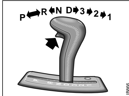
Detent positions for selector movement
