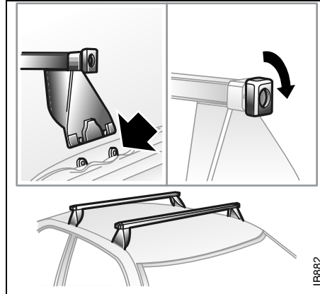
Mounting holes for load carrier, front on Coupés and front/rear on five-door models
