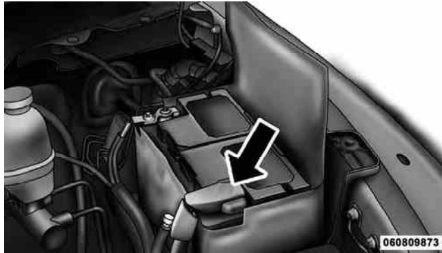
Positive Battery Post
