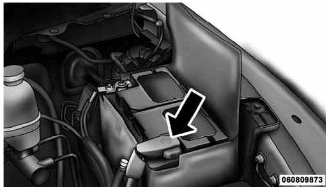
Positive Battery Post
