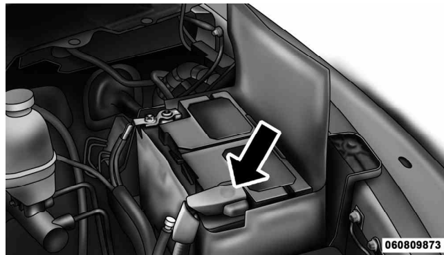
Positive Battery Post
