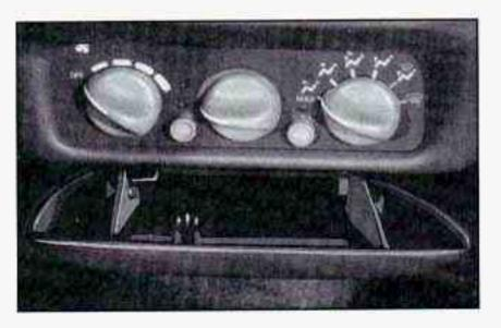
For the instrument panel ashtray, open it, push down on the locking tab and pull out the ashtray.
