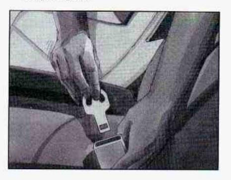
You can make the belt longer by tilting the buckle and pulling it along the belt.
