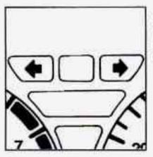
A green arrow on the instrument panel will flash in the direction of the turn or lane change.
