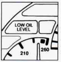
Your engine is equipped with an oil level monitoring system. When the ignition key is turned on, the LOW OIL LEVEL light will briefly flash. If the light does not flash, have it fixed so it will be ready to warn you if there's a problem.
