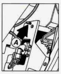
If the pointer isn't at 0 (zero), turn the horizontal aiming screw to adjust the aim. Check the vertical aim indicator. The bubble should be centered on 0 (zero).
