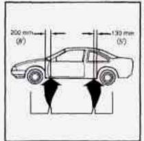
Position the jack under the vehicle and raise the jack lift head until it fits firmly into the notch in the vehicle's frame nearest the flat tire.
