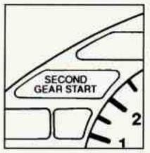
The SECOND GEAR START light on the instrument cluster will come on when this feature is active.
