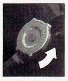
You can remove the radiator pressure cap when the cooling system, including the radiator pressure cap and upper radiator hose, is no longer hot. Turn the pressure cap slowly to the left until it first stops. (Don't press down while turning the pressure cap.)
