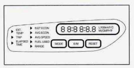
When you start your engine, the trip calculator will display a mode. A lighted arrow shows which mode is displayed.
