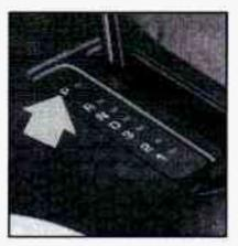
Your automatic transaxle may have a shift lever on the steering column or on the console between the seats.
