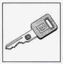
Your vehicle is equipped with the PASS-Key II (Personalized Automotive Security System) theft deterrent system, PASS-Key II is a passive theft deterrent system. This means you don't have to do anything different to arm or disarm the system.
