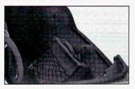
Your vehicle may have a convenience net. You'll see it on the back wall of the trunk. Put small loads, like grocery bags, behind the net. It can help keep them from falling over during sharp turns or quick starts and stops.
