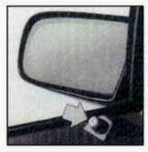
The electric mirror control is near the driver's window. Turn the control to the left to adjust the left mirror or to the right to adjust the right mirror. Then move the control in the direction you want to move the mirror.
