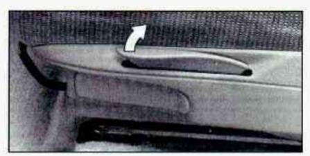
Lift the lever to release the seatback, then move the seatback to where you want it. Release the lever to lock the seatback in place. Pull up on the lever without pushing on the seatback, and the seatback will move forward.
