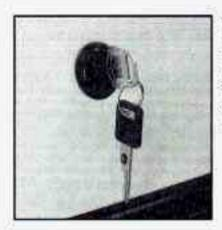
To unlock the trunk from the outside, insert the door key and turn it. You can also use the Remote Lock Control, if your vehicle has this option.
