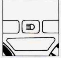
To change your headlamps from low beam to high beam, or high to low, pull the multifunction lever all the way toward you. Then release it. When the high beams are on, a blue light on the instrument panel also will be on.
