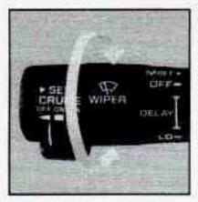
You control the windshield wipers by turning the band marked WIPER. For a single wiping cycle, turn the band to MIST. Hold it there until the wipers start, then let go. The wipers will stop after one cycle. If you want more cycles, hold the band on MIST longer.
