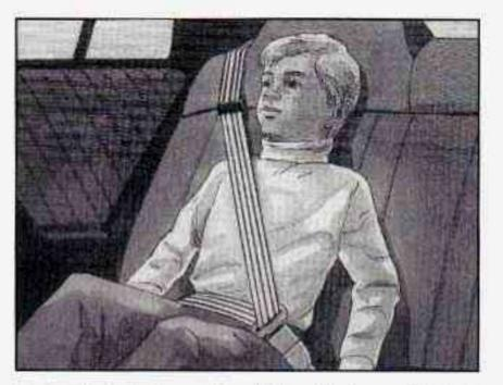
Buckle the belt around the child, and make sure that both the lap belt and the shoulder belt are secured properly. Make sure that the shoulder belt crosses the shoulder, See "Safety Belts, Rear Seat Passengers" in the Index.
