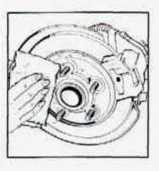
Remove any rust or dirt from the wheel bolts, mounting surfaces and spare wheel. Place the spare on the wheel mounting surface.
