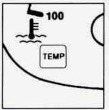
This light tells you that your engine coolant has overheated or your radiator cooling fan is not working.
