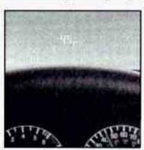
If you have the Head-Up Display (HUD), you can see the speedometer reading, in English or metric units, displayed "through" the windshield. The HUD also shows these lights when they are lit on the instrument panel:
