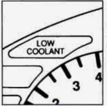
If this light comes on, your system is low on coolant and the engine may overheat. See "Engine Coolant" in the Index and have your vehicle serviced as soon as you can.
