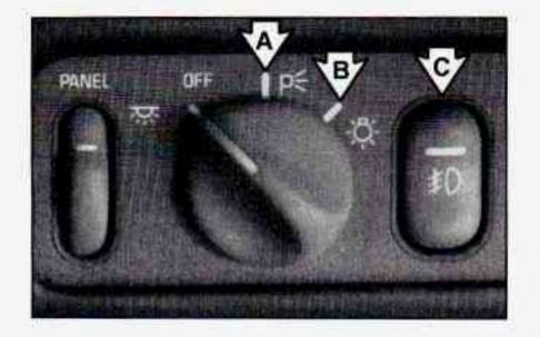
Turn the knob to LAMPS (B) to turn on the headlamps and other operating lamps.
