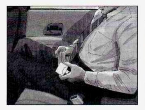
When you sit in a center seating position, you have a lap safety belt, which has no retractor. To make the belt longer, tilt the latch plate and pull it along the belt. To make the belt shorter, pull its free end as shown until the belt is snug.
