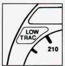
When your anti-lock system is adjusting brake pressure to help avoid a braking skid, the LOW TRAC light will come on.
