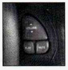
You can control certain audio system functions using the buttons on your steering wheel. **VOLUME:** Press the up or down arrows to increase or decrease volume.
