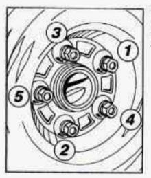
Tighten the wheel nuts firmly in a crisscross sequence as shown.
