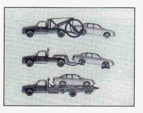
Use wheel lift or car carrier equipment. Additional ramping may be required for car carrier equipment. Use safety chains and wheel straps.
