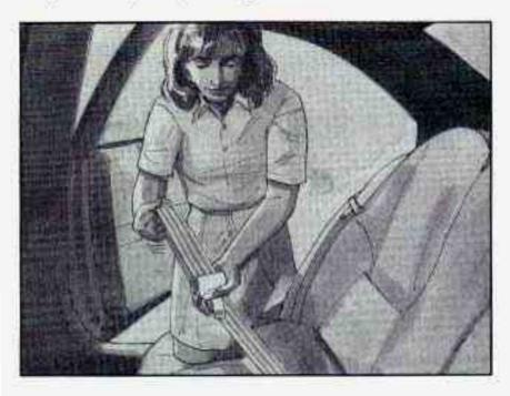
Put the restraint on the seat. Follow the instructions for the child restraint.
