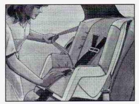
To tighten the belt, feed the shoulder belt into the retractor while you push down on the child restraint.
