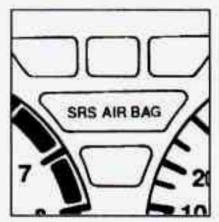
You will see this light flash for a few seconds when you turn your ignition to RUN or START. Then the light should go out. This means the system is ready.
