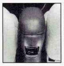
To remove the rear console ashtray, open it, push down on the snuffer and pull the ashtray out of the console. To remove the rear door ashtray, open and pull up on the ashtray door.
