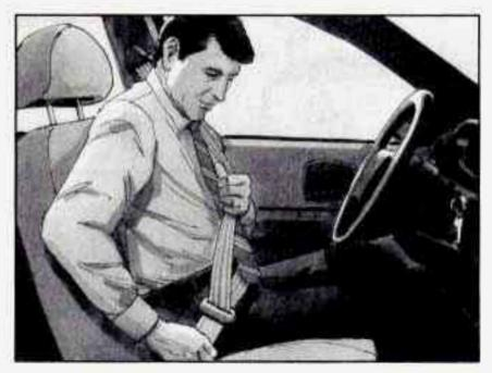
To make the lap part tight, pull down on the buckle end of the belt as you pull up on the shoulder belt.
