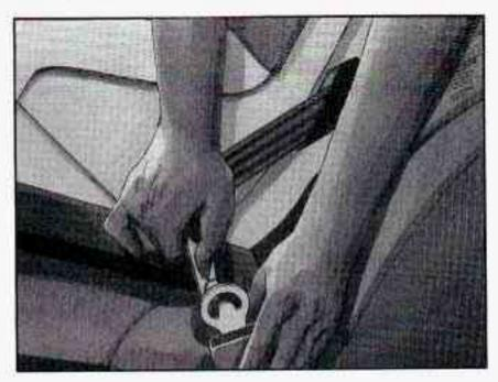
To make it tight, pull the belt while you push down on the child restraint. If the belt won't stay tight, switch it end for end.
