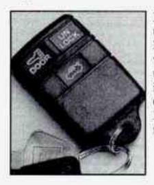
Press UNLOCK once to unlock the driver's door. Press UNLOCK again within five seconds to unlock all the doors. The interior lamps will come on (see "Sustained Interior Illumination" in the Index for more details).
