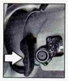
A tilt steering wheel allows you to adjust the steering wheel before you drive. You can also raise it to the highest level to give your legs more room when you exit and enter the vehicle.
