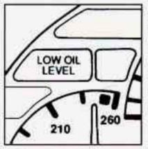
If the LOW OIL LEVEL light on the instrument panel comes on, it means you need to check your engine oil level right away. For more information, see "Low Oil Level Light" in the Index.
