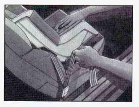
Push and pull the child restraint in different directions to be sure it is secure.
