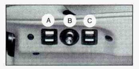
FRONT (A): Raise the front of the seat by holding the switch up. Hold the switch down to lower the front of the seat.
