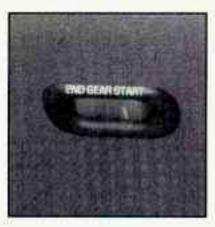
Your vehicle may be equipped with a Second-Gear Start feature. The button is below the lamp controls.
