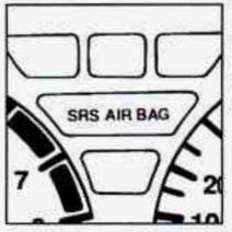
There is an air bag readiness light on the instrument panel, which shows SRS AIR BAG or the air bag symbol.
