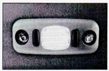
The dome lamp will go on when you open the doors. Next to the dome lamp are two reading lamps. Turn them on using the switches.
