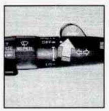
At the top of the multifunction lever. there's a paddle with the word PUSH on it. To spray washer fluid on the windshield, push the paddle. The wipers will run for several sweeps and then either stop or return to your preset speed.
