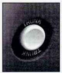
Press the button behind the glove box door to unlock the trunk from inside your vehicle. Your transaxle shift lever must be in PARK (P).
