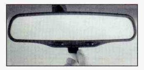
To reduce glare from lamps behind you, move the lever to the night position.
