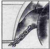
Attach T-hook chains in front of the wheels into the side slots of the cradle on both sides.
