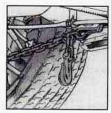
Attach T-hook chains into the slotted holes in the bottom of the floor pan support rails just ahead of the rear wheels on both sides.
