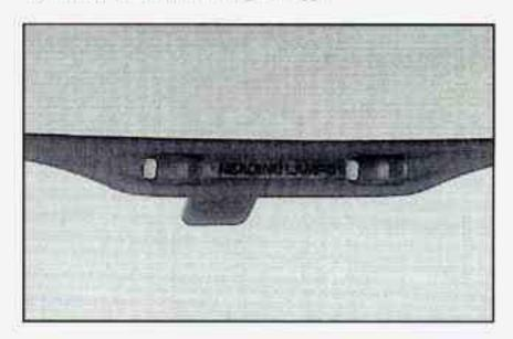
These lamps go on when you open the doors. When the doors are closed, turn them on and off with the switches.
