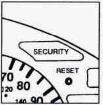
This light will come on when you turn the key to START and stay on until the vehicle starts. It will also come on and stay on if your key is too dirty or wet for the PASS-Key<sup>®</sup>II system to read the resistor pellet.
