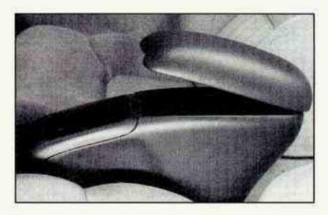
To open the storage area, press the latch on the front edge and pull up. The console has a cupholder, cassette tape storage and a coinholder.
