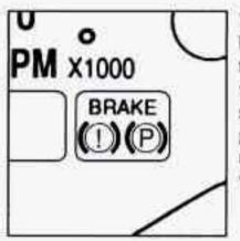
Your Pontiac's hydraulic brake system is divided into two parts. If one part isn't working, the other part can still work and stop you. For good braking, though, you need both parts working well.
