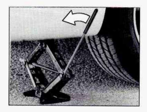
Lower the vehicle by turning the jack handle counterclockwise. Lower the jack completely.
