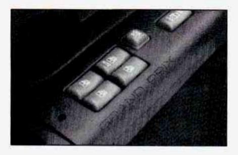
Switches on the driver's door armrest control each of the windows when the ignition is on. In addition, each passenger door has a switch for its own window. The driver's window switch has an auto-down feature. This switch is labeled AUTO. Tap the rear of the switch, and the driver's window will open a small amount. If the rear of the switch is pressed all the way down and released, the window will go all the way down.
