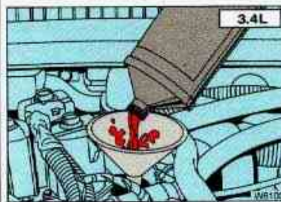
Twin Dual Cam 3.4L V6: Adding Automatic Transaxle Fluid
