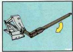
If your wheel has the special locking lug nut, use the special adapter supplied with your vehicle to remove the locking wheel nut by turning counterclockwise. Use the wheel wrench to loosen the wheel nuts, but don't remove them. Attach the wheel wrench to the jack, and rotate the wrench clockwise to raise the jack head a few inches.
