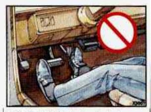
Don't "ride" the brakes by letting your left foot rest lightly on the brake pedal while driving.
