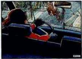
You can steer around the obstacle while braking hard. As you brake, your computer keeps receiving updates on wheel speed and controls braking pressure accordingly.
