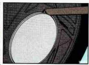
6. If you have aluminum wheels, remove the center cover that conceals the wheel nuts by using the flat end of the wheel wrench to pry it off. Do not drop the cover or lay it face down, as it could be scratched or damaged.
