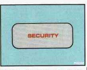
The ignition key must be clean and dry before it's inserted in the ignition or the engine may not start.
