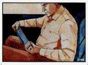
When you sit in a center seating position, you have a lap safety belt, which has no retractor.
