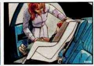
Pull the rest of the lap belt all the way out of the retractor to set the lock.
