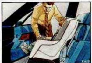
To tighten the belt, feed the lap belt back into the retractor while you push down on the child restraint. Push and pull the child restraint in different directions to be sure it is secure. To remove the child restraint, just unbuckle the vehicle's safety belt and let it go back all the way. The safety belt will move freely again and be ready to work for an adult or larger child passenger.
