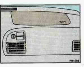
Your Pontiac may have the right-front passenger's SIR option. If your vehicle has an air bag for the right-front passenger, it will say SIR on the instrument panel above the glove box. Here are the Most Important Things to Know:
