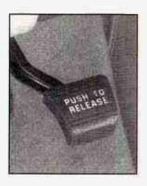
The parking brake is located on the driver's side under the instrument panel.
