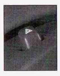
Your hazard warning flashers button is located on top of the steering column.
