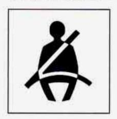
When the key is turned to RUN or START, a chime will come on for about eight seconds to remind people to fasten their safety belts, unless the driver's safety belt is already buckled. The safety belt light will also come on and stay on until the driver's belt is buckled.
