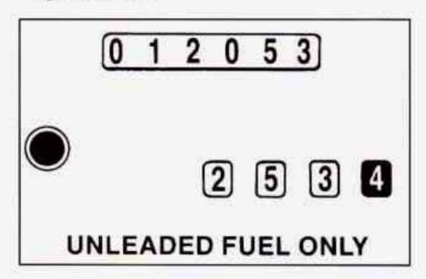
The trip odometer can tell you how far your vehicle has been driven since you last set it to zero. To set it to zero, push the reset button located above the fuel gage.
