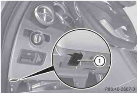
Hood release lever in driver's footwell
