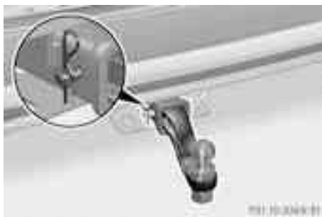
Correctly installed and secured ball coupling
