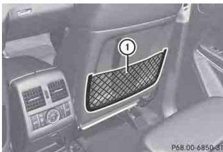
① Storage net on the back of the front seats
