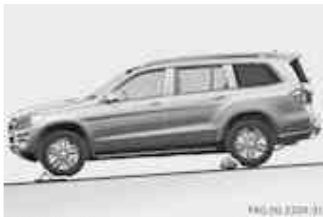
Securing the vehicle on slight downhill gradients
