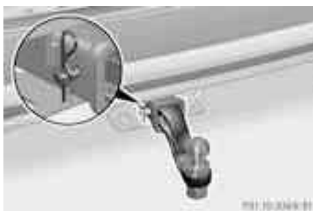
Correctly installed and secured ball coupling
