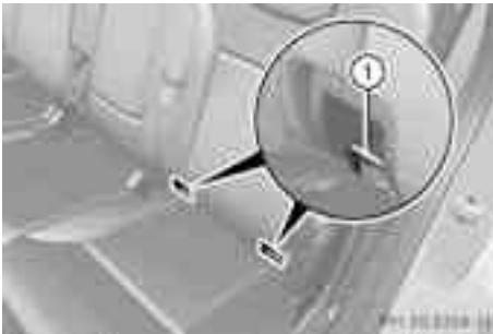
Securing rings for the outer seats in the second row
