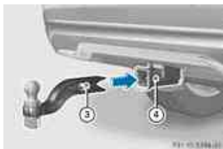
Hole in the ball coupling and ball coupling recess
