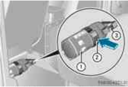
Fire extinguisher (vehicles with a stowage compartment)
