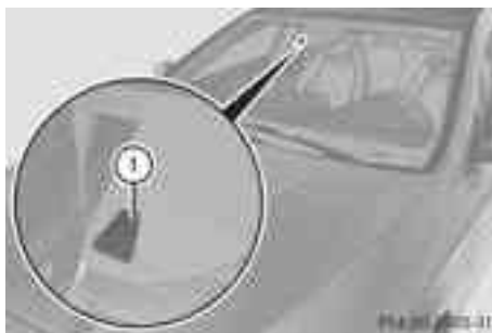
① Speed Limit Assist camera
