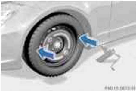
Positioning a wheel (example: vehicle with an emergency spare wheel)
