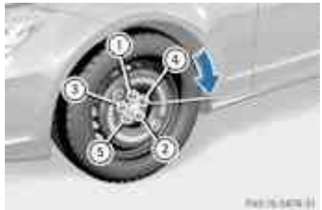
Tightening the wheel nuts (example: vehicle with an emergency spare wheel)
