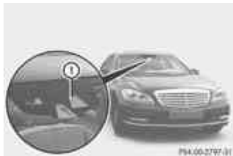
① Speed Limit Assist camera
