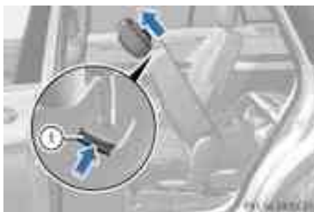
Removing the head restraints from the outer seats in the 2nd row of seats
