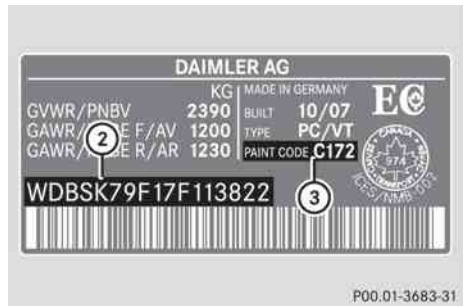
Example: vehicle identification plate (Canada only)
