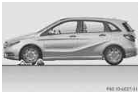
Securing the vehicle on level ground
