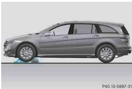
Securing the vehicle on level ground
