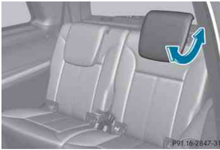
Head restraints on the outer seats in the 3rd row of seats
