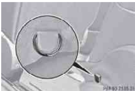
Cargo tie-down rings, third-row footwell
