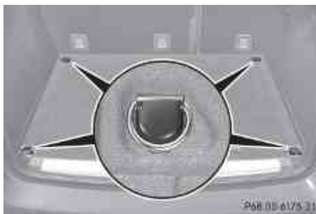
Cargo tie down rings, cargo compartment
