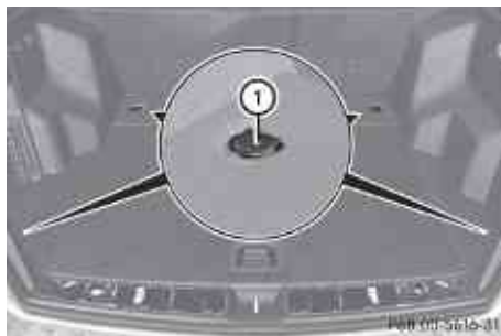
Cargo tie-down rings, cargo compartment
