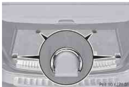
Cargo tie down rings, cargo compartment
