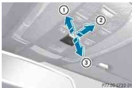
Roof panel switch
