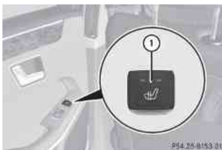
Rear seat heating switch (Canada only)
