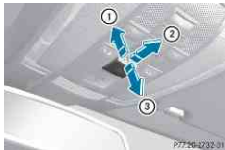
Roof panel switch
