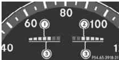
Front area warning indicators
