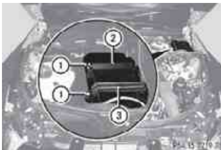
Fuse box on driver's side
