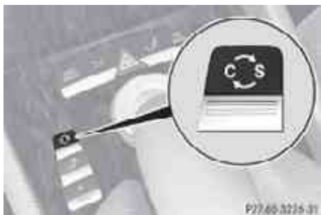
Program mode selector switch
