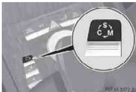
Program mode selector switch on AMG vehicles
