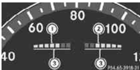
Front area warning indicators
