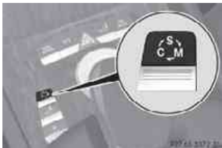
Program mode selector switch on AMG vehicle
