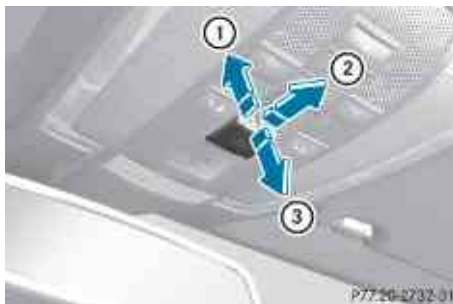
Roof panel switch
