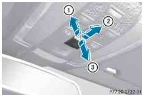
Roof panel switch
